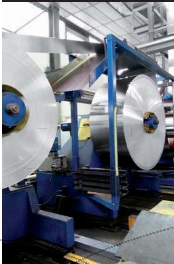
1 A - Uncoiler B - Strip joiner
