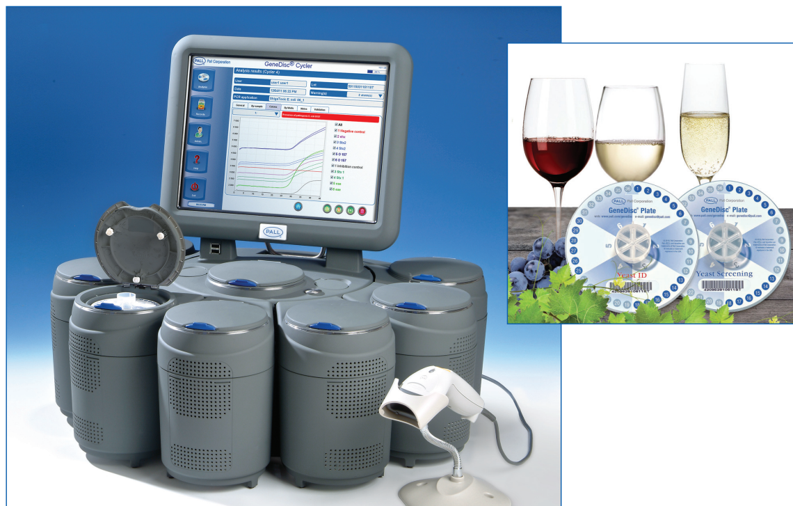
Figure 1: The GeneDisc System including the GeneDisc Cycler and GeneDisc Plate
