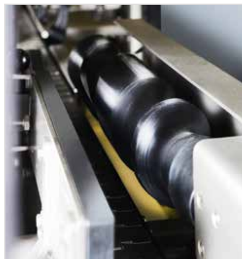
Coclea universale per contenitori cilindrici, variazione 40-70 mm e 70-110 mm Universal screw feeder for cylindrical contain- ers, variation 40-70 mm and 70-110 mm
