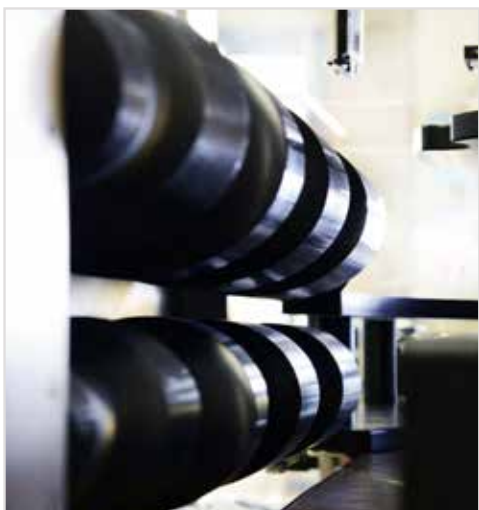
Doppia coclea sovrapposta per contenitori instabili Dual overlapping screw feeder for unstable containers
