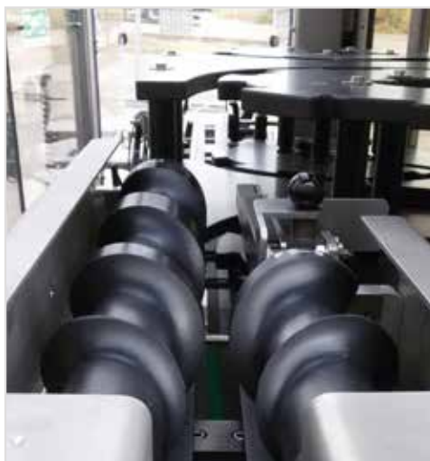
Doppia coclea contrapposta per contenitori sagomati Dual opposing screw feeder for shaped containers
