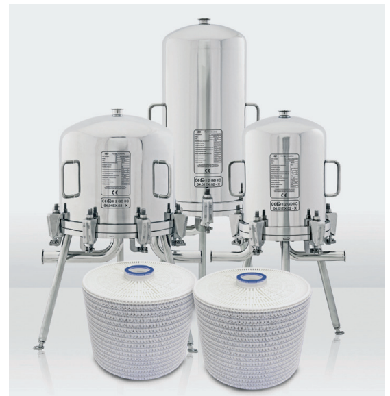
Figure 3: Pall's WSFZ housings for SD II modules provide flexibility in production. By installing internal center posts of different lengths, filtration can be run at 25, 50, 75 and 100% of capacity. Special adaptors enable retrofitting with SUPRApak modules as production capacity increases.
